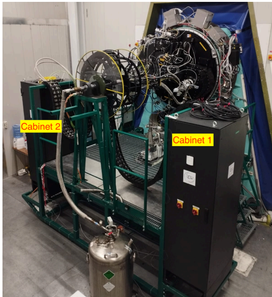
Figure 1: The SOXS spectrograph installed at the Nasmyth focus of the ESO-NTT.
