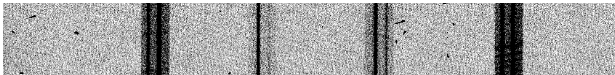
Figure 50: Acquisition image (SOXS.2025-10-22T04:50:55.102.fits) and UV-VIS spectrum (SOXS.2025-10-22T04:51:52.337.fits) of two stars with an angular separation of 4.1'' , both placed along the 1'' slit (position angle = -86.3 deg). The measured separation between the two spectral traces in each order is 14.9 pixels, resulting in a plate scale of 0.28''/\text{pixel} .
